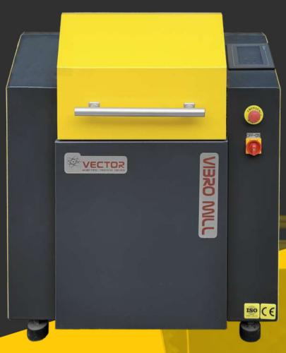
Special soundproofed safety cabin. It is used in the grinding process of fragile materials and minerals such as basalt, bauxite, concrete, chrome, vanadium, dolomite, ferromanganese, ferrovanadium, granite, coal, quartz, silicate, limestone, slag.
