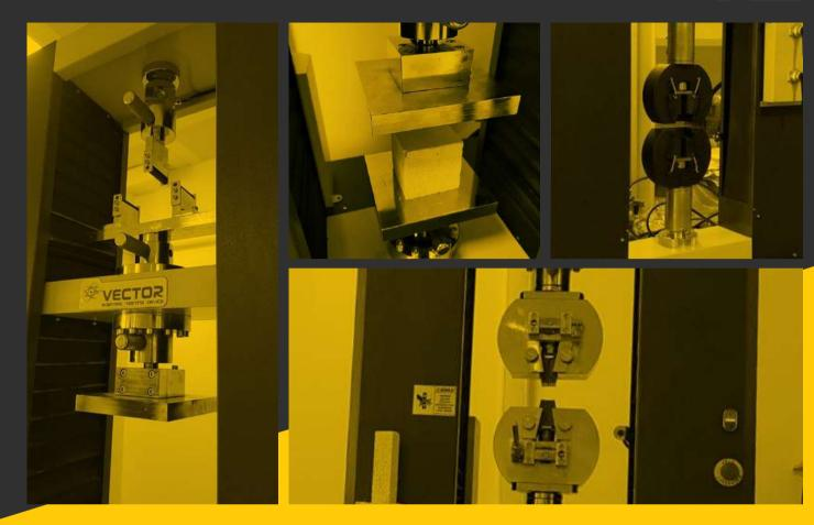
Standards: ISO 7500-1, ASTM E4, DIN 51221. AFNOR A03-501, TS EN ISO 6892-1, TS 1398-1 EN ISO 527-1, TS FN ISO 178: 2010.
